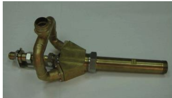
Figure 4 – Photographs of various ejectors tested with different low-boiling refrigerants
